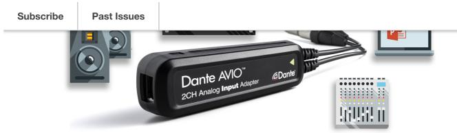
Audinate have announced a range of <u>stereo Dante adaptors</u>, to quickly bring stereo devices onto a network. They will be available in stereo analogue input, analogue output, AES in & out, and USB class-compliant configurations, although they do require Power-over-Ethernet to function.
