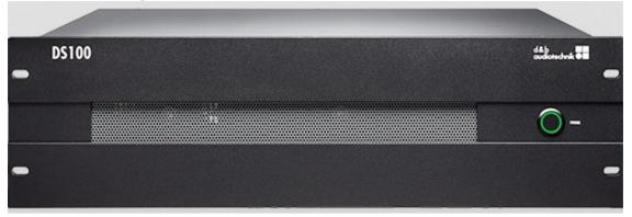
d&b audiotechnik have announced their <u>Soundscape</u> system, which combines a 64x64 level and delay matrix with software. The En-Scene software is a sound object positioning tool to place up to 64 inputs in a three dimensional space; whilst En-Space is a room reverb emulation package allowing modification of room reverbs.
