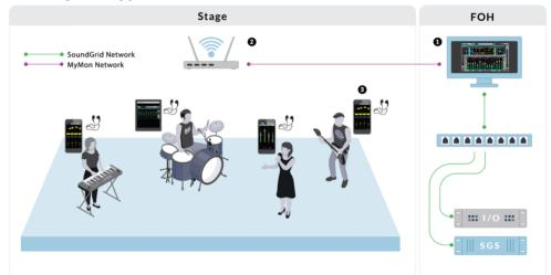
The MyMon app runs in conjunction with the Waves LV1 system. It allows the user to remotely access levels, EQ and pan. Up to 16 devices can be added at once. Find out what PSN Europe thought <u>here</u> and read about the LV1 <u>here</u>. You can also download the app for android and iOS <u>here</u>.
